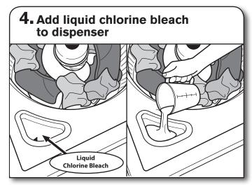
Do not overfill, dilute, or use more than 1 cup (236 mL). Do not use color-safe bleach or Oxi products in the same cycle with liquid chlorine bleach.
